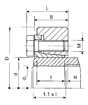
B mm = 57.5 d H8 mm = 135 D mm = 230.0 ds mm = 95 F kN torque = 387
